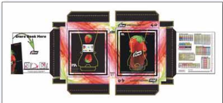
2.4a: Profiled Contract Proof: The contract proof must include a control target as well as template layout markings.
