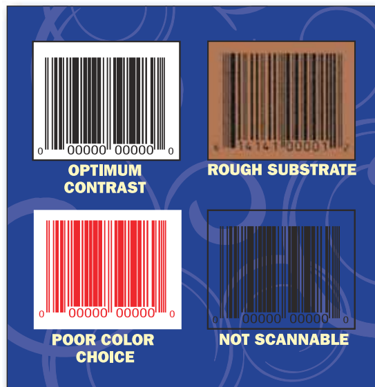
3.3.2b: Color Considerations: The optimum bar code color combination is opaque black ink for the bars and opaque white substrate or ink for the background.
