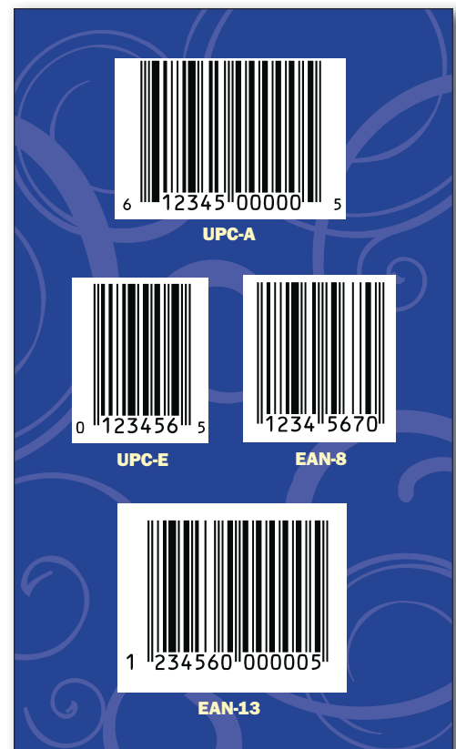
3.3.2a: Bar Code Type: The type of bar code depends on many factors including where it will be scanned and how it will be printed.
